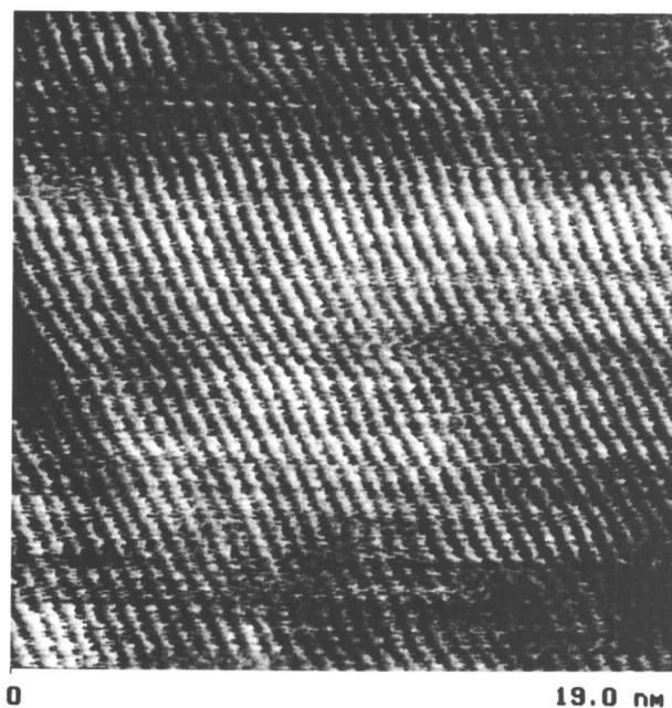
Figure 2. LFM image of oriented PTFE obtained with a -\text{CF}_3 tip in ethanol ( z = 0.1 \text{ V} ). Molecular resolution is a result of a stick-slip process.
